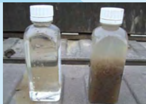
MBR Effluent vs. Raw Sewage
